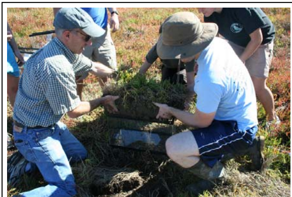
David Sedlak and Patrick Ulrich collect wetland microcosm cores from a tidal salt marsh along the Petaluma River.
