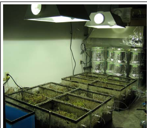
Experimental setup for laboratory wetland microcosm operation.
