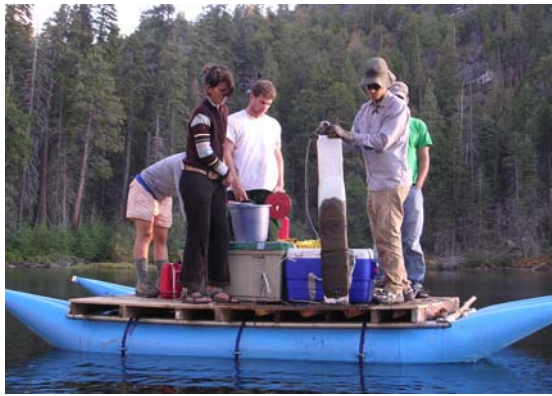
Researchers collecting a frozen sediment core from Swamp Lake, September 2006.
