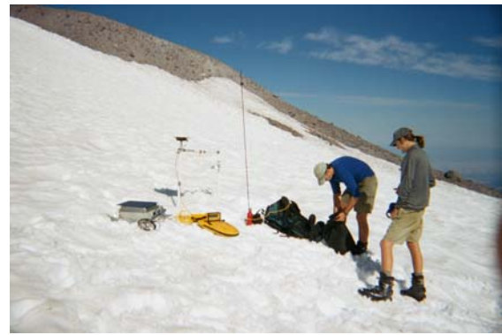
Field work on the Hotlum Glacier, showing echo sounder equipment and GPS position recording.
