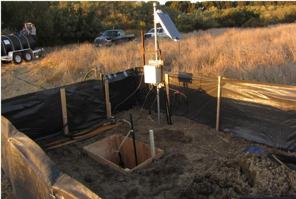
Figure 1. Site configured for infiltration testing, Monterey County.
