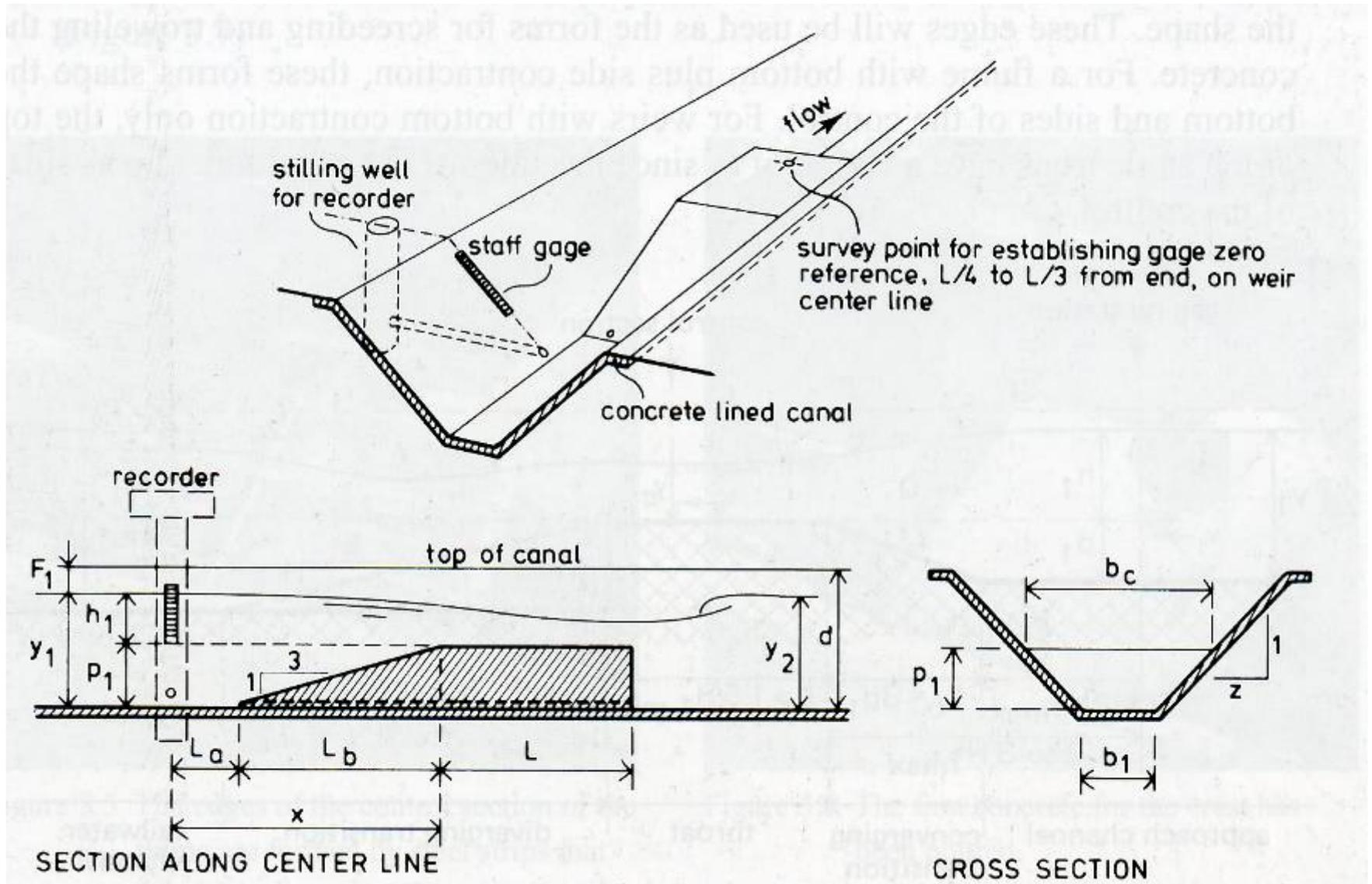
In these flumes, throats are so long that streamlines are parallel in a short distance of throat section and energy equation can be applied through gaging and throat sections.
